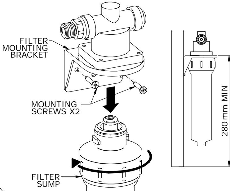
First you will need to remove the filter sump. This can be done by turning the sump a quarter turn clockwise and pulling down.
